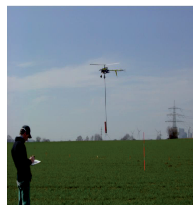
Figure 3: Autonomous UAS flight during the aeromagnetic survey near Cologne.
