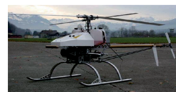
Figure 4: Scout B1-100. Developed by Aeroscout GmbH, Switzerland. Weight 43 kg. Payload 18 kg.
