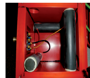
Figure 8: VLF/LF sensor – consisting of three perpendicular coils.
